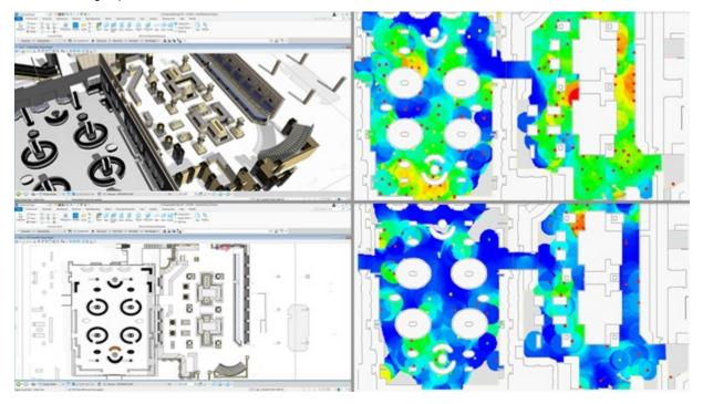
Top left illustrates a 3D model of a retail operation created using OpenBuildings Station Designer. Bottom left shows 2D floor plans that are then imported into LEGION Simulator (right) to test two scenarios. Examples shown are at occupancy rates of 75% (top) and 25% (bottom) to comply with social distancing requirements.
